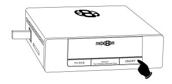
Power Up and hold on/off button for 10 seconds
