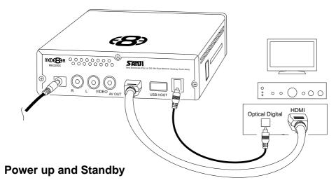
Plug the AC/DC adapter into the mains outlet and plug the DC Jack into the DC IN at the rear of the MED200X. **DO NOT USE ANY AC/DC ADAPTER AND ONLY USE THE ONE SUPPLIED** otherwise you may cause damage to the unit. Press the On/ Off button on the Mede8ers front panel and front facia LED will turn on Blue. You can put your Mede8er into standby by pressing the On/Off button on the remote. When in standby the front facia LED will turn Red.
