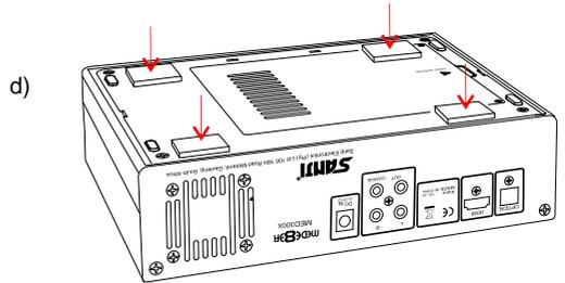
Make sure that the DC cable is unplugged. Turn the Mede8er upside down and unscrew the hard drive cover screws x and y. Lift the hard drive cover and remove it, place it on a flat surface with the mounting tabs facing upright. Fit a compatible SATA hard drive into place with the label facing upwards and the connectors facing the side with the air vents. Secure the hard drive with the four screws provided.
