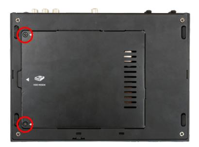
Unplug the all cables into the MED500X2 and turn it upside down. Unscrew the two star screws as indicated by the red circle on the image on the left.
