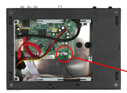
Disconnect the fan connector as indicated in the image on the left. Replace the cover plate and insert and tighten the screws.
