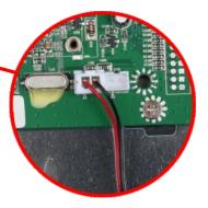
**WARNING** - If you install an internal Hard Drive at a later stage please remember to reconnect the fan connector.
